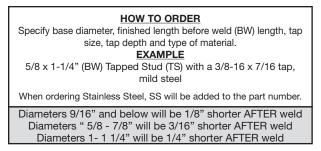
**Tapped Studs** are used in all types of applications. They can be welded to a flat surface, or to the inside or outside of an angle.
